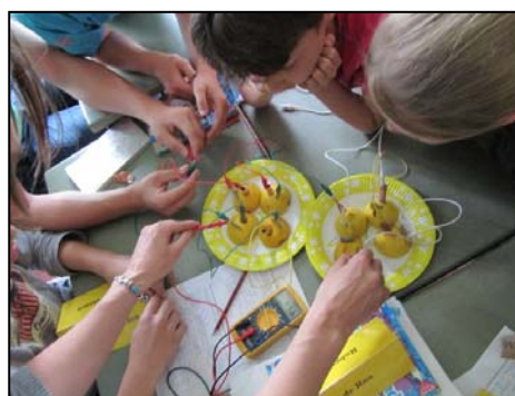
Making a lemon battery for a LED light
